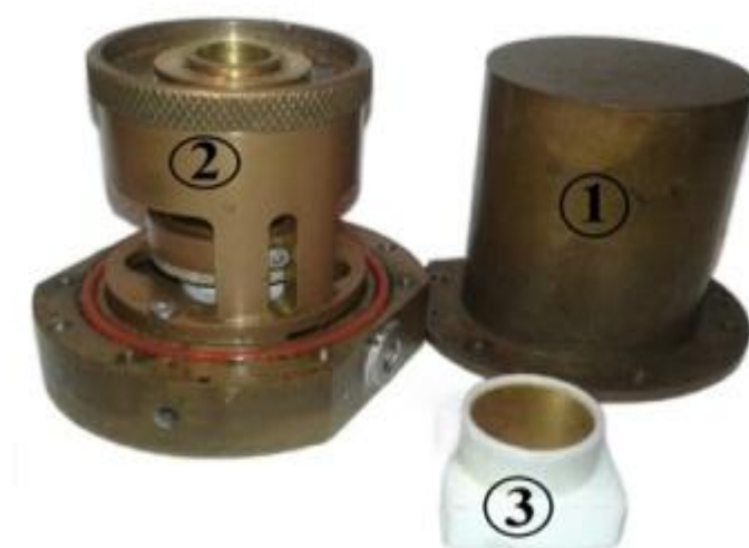
Fig. 4.3. Measuring holder (No.2) with gas-tight screwed lid (No.1) and electrode in Teflon cover (No.3).
