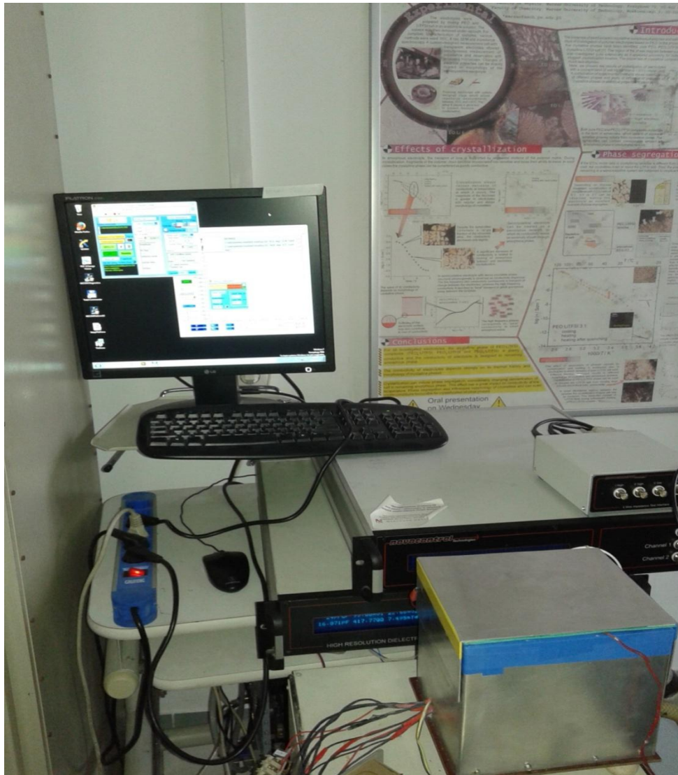
Fig. 4.5. The measuring system for impedance spectroscopy.
